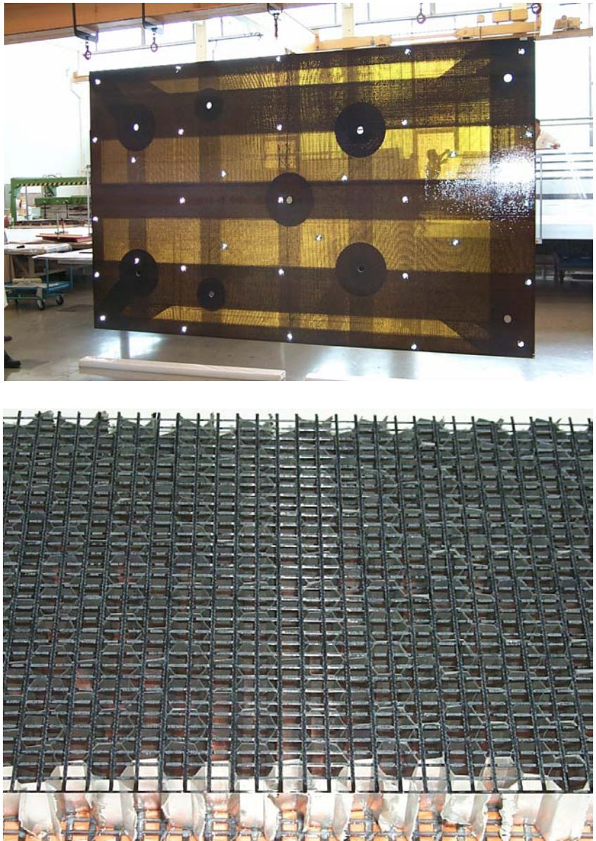
Figure 14 – ultra-lightweight design of a solar panel (source: Eurocopter)
