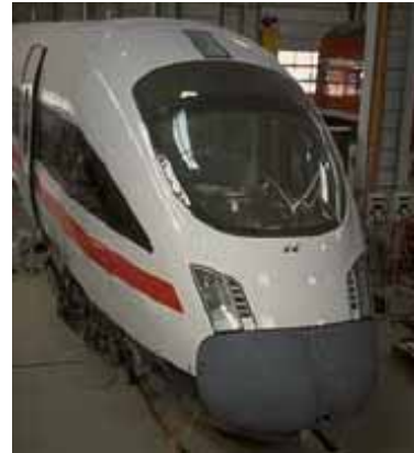
Composite high speed train cab produced by VI (courtesy of Alcan Airex Composites)
