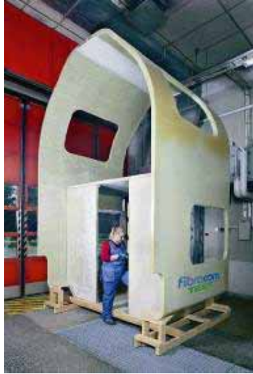
A prototype composite double-deck coach section, providing a 20% weight saving over aluminium (courtesy of Fibrocom)
