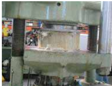
Compression testing of an energy cell component from a prototype all-composite structural cab design
