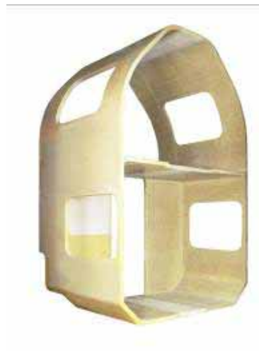
A prototype lightweight composite double-deck coach section (courtesy of Fibrocom)
