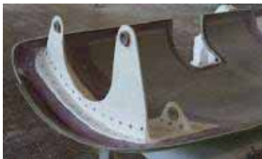
A hybrid bolted-bonded T-joint between the external cover and bracket of a composite sandwich coupler door for the Italian ETR 460/470/480 high speed train (courtesy of Sistema Compositi and the University of Rome)
