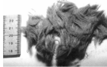
Glass fibres recovered using a fluidised bed process (courtesy of the University of Nottingham)
