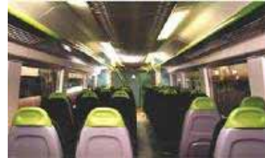
Fire safe composite interior components (moulded with aluminium hydroxide-filled polyester resin) for the Electrostar trains (UK) (courtesy of DSM Composite Resins)
